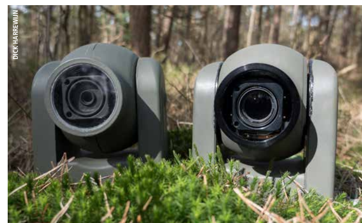
The Bradley (BR Remote) CamBall 3 was used for filming buzzards on their nest. On the right is the original camera, on the left the 3D printed dummy camera
