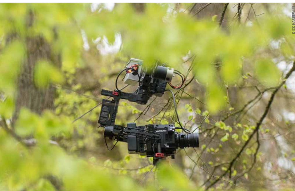
At the end of the production we were able to use the VariCam LT in combination with a Ronin for cable-cam shots
